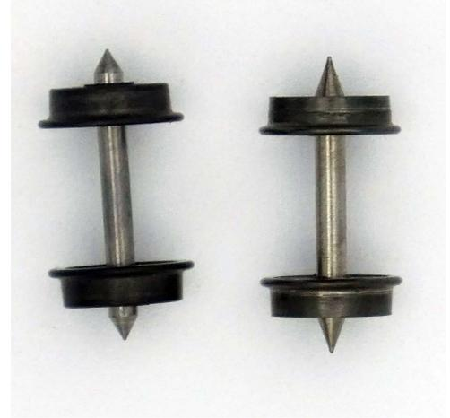
*Old style wheels on left, reamers are designed for use with these. Modern longer axles on right.*
